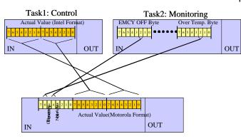
The relationship between variables of two different process images (done at configuration time) defines a mapping object, describing all relations between variables of the process images. A process image shares exact one mapping object with every other process image in which linked
