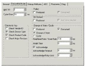
The CANopen Node and PDO configuration of the Beckhoff FC510x CANopen cards can be done manually – this allows to connect devices that do not have Electronic Data Sheets (eds) Files available. Alternatively eds based configuration is possible as soon as CiA-WD306 is in place.
