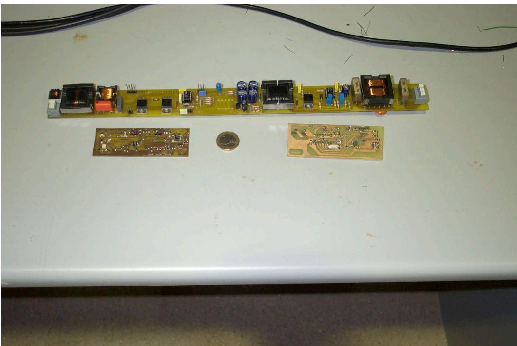
Figure 8: Photo of the 3 boards (ballast/base, CAN and protection circuits).
