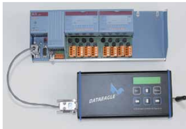
Figure 2: DE 6000 with a controller of Bernecker + Rainer coupled to a S7 PLC
