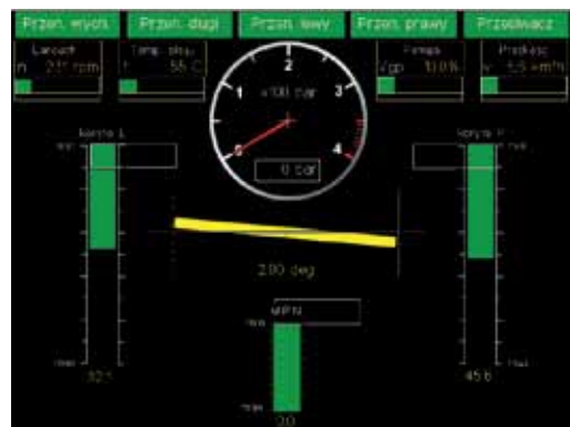
Figure 7: Display in the operator's cabin (screen for chain leveling)
