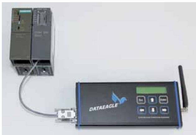
Figure 1: DE 6000 used with a CAN module by Helmholz on a S7 PLC
