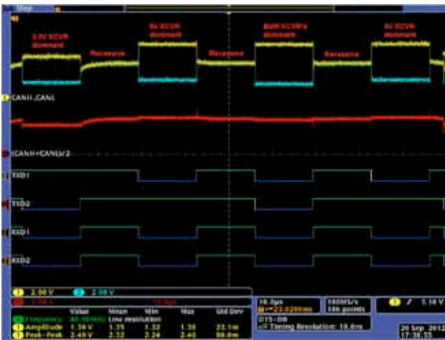
Figure 8: Waveforms of a 5-V SN65HVD255 and a 3,3-V SN65HVD234
