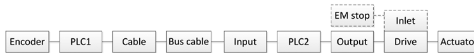
Figure 2: The safety block diagram of structure A, where one of the encoders initiates the stopping function.
