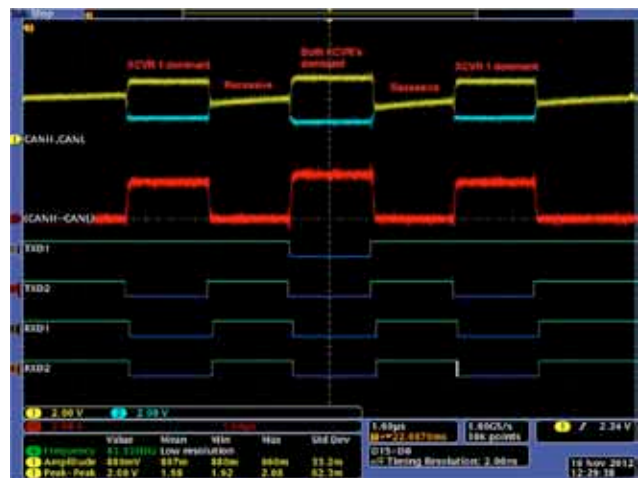
Figure 5: Waveforms of two 3,3-V SN65HVD234 transceivers by Texas Instruments
