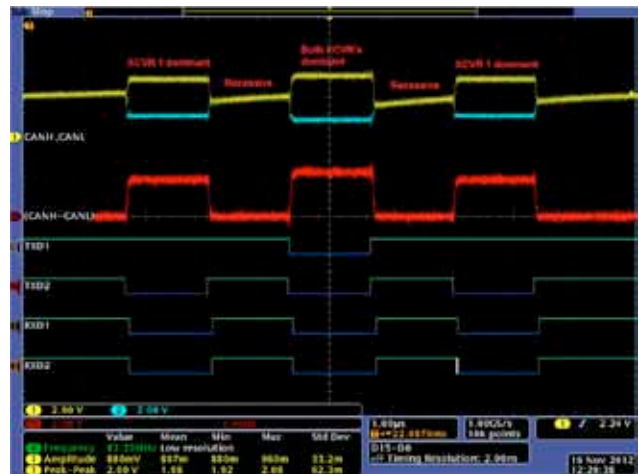
Figure 6: Waveforms of two SN65HVD255 transceivers, one with a +1-V ground shift
