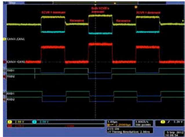
Figure 4: Waveforms of two 5-V SN65HVD255 transceivers by Texas Instruments
